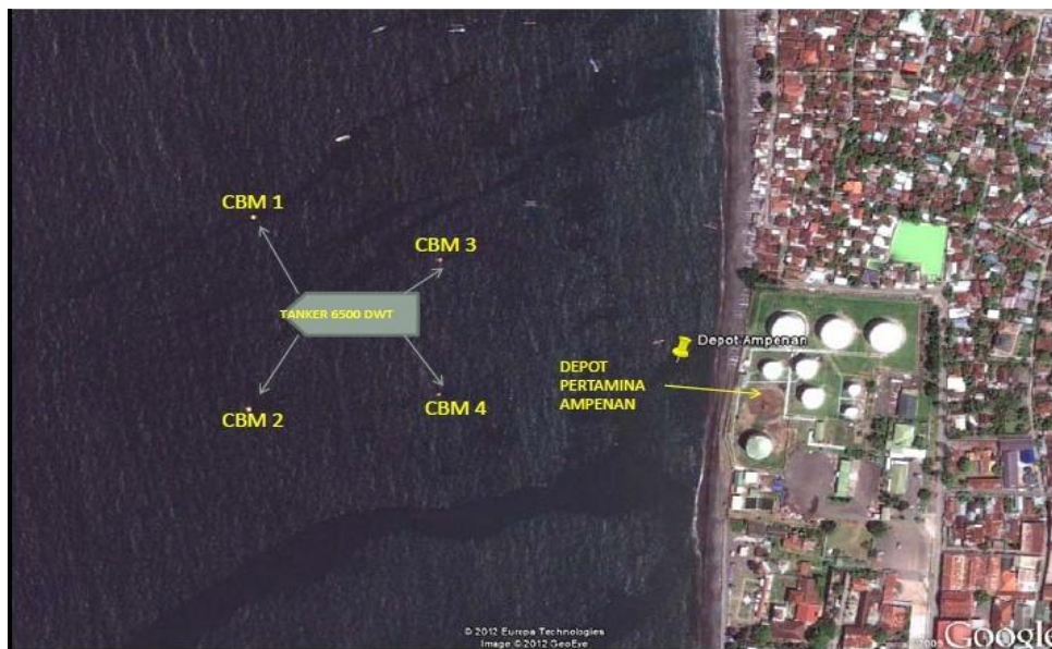
Gambar 1.1 Lokasi Sistem Conventional Buoy Mooring
