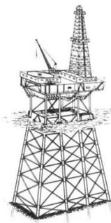
Gambar 1 Ilustrasi jacket platform
